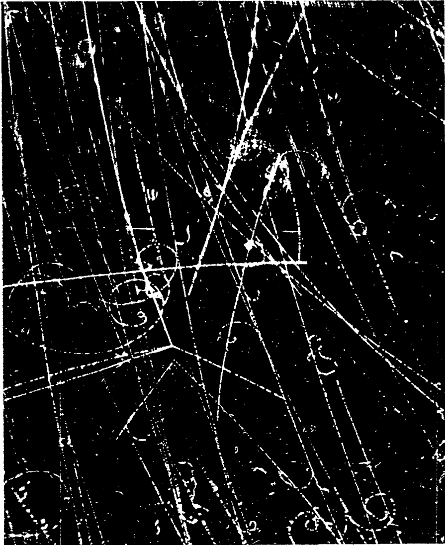
Fig. 5. Annihilation of an antiproton in carbon giving rise to a K meson and a \Lambda hyperon.
