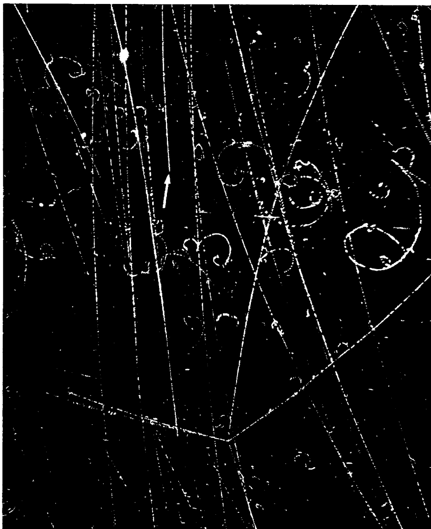
Fig. 1. An antiproton enters a propane bubble chamber, and at the point marked with an arrow undergoes charge exchange. The antineutron originates the annihilation star (directly below). Density of propane 0.42 \text{ g/cm}^3 . Real distance between charge exchange and origin of star 9.5 \text{ cm} . T_{\bar{p}} at charge exchange \sim 50 \text{ MeV} . (From Agnew et al. 6 )
